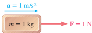
Fig. 1.2 A force of 1 newton applied to a body of mass 1 kg provides an acceleration of 1 m/s 2 .
